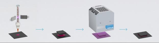
Dispensing and irradiation in one step with DELO-ACTIVIS Joining
